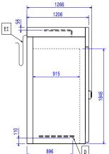
Electrical inlet (power) ΕI Refrigerant Outlet
